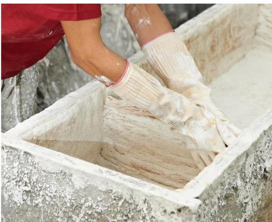
We have rediscovered constructive materials. Cement, sand and granite, reinforced with the natural fiber Ramie.
