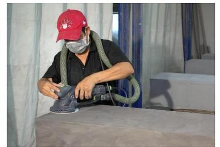
Sanding the surface of the raw cement is the first step. The pigment is applied by hand, giving each piece the individual touch. After the pigmented surface dried, the loosen pigment is taken of.
